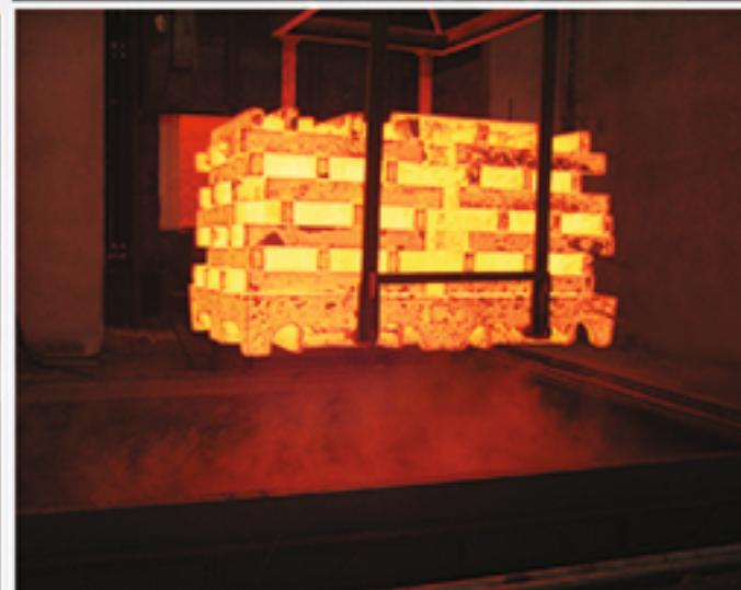
1 Computer Controlled electrical heat treatment furnace capacity of 10 tones
